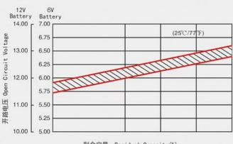
剩余容量 Residual Capacity(%) Open Circuit Voltage vs Resideual Capacity
